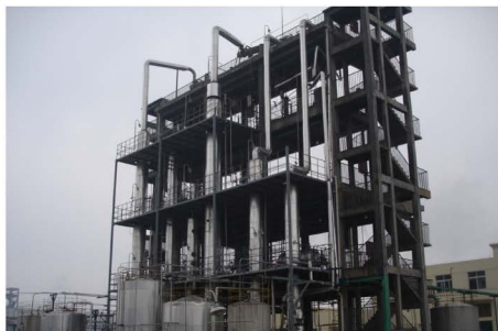
Fig. 10. Ti-MWW-based innovative MEK ammoxidation process and 15,000 t/y MEKO plant (China).
